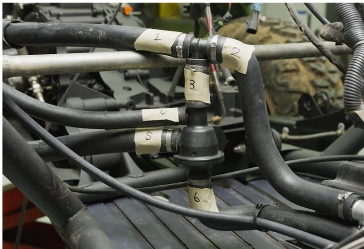
**4. Remove 4 main hoses and coolant tank small hose, remove thermostat housing, vertical hose and upper T fitting and discard.**
