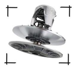
NOTE: No component marking is required before disassembly. The clutches feature factory apposed index marks as references if needed.
