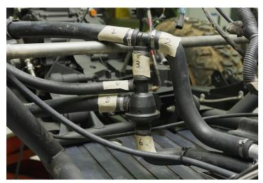
4. Remove 4 main hoses and coolant tank small hose, remove thermostat housing, vertical hose and upper T fitting and discard.
